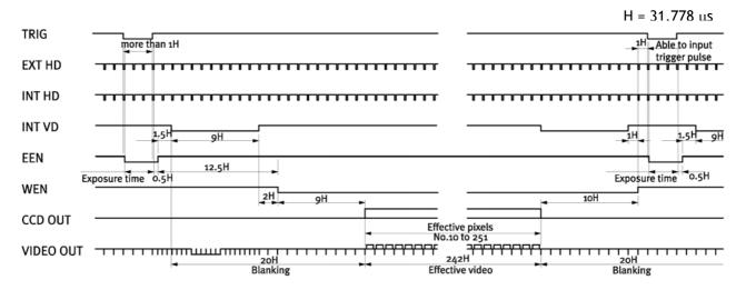
Fig. 15. Vertical timing for pulse width control
